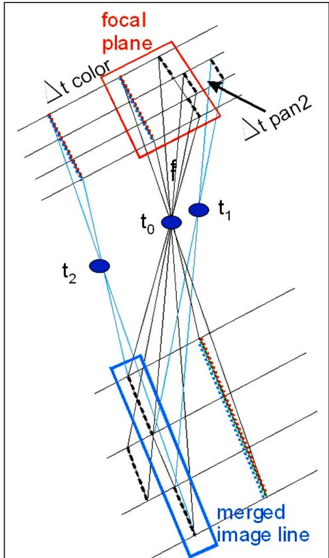
Fig. 3: combination of CCD-sensors with different location in the focal plane to a homogenous synthetic CCD-line
