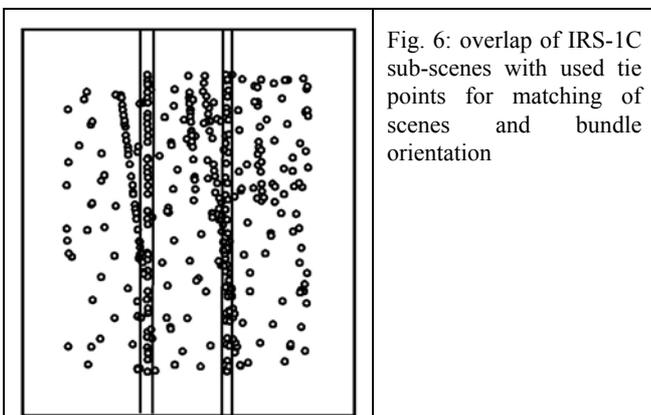
Fig. 6: overlap of IRS-1C sub-scenes with used tie points for matching of scenes and bundle orientation
