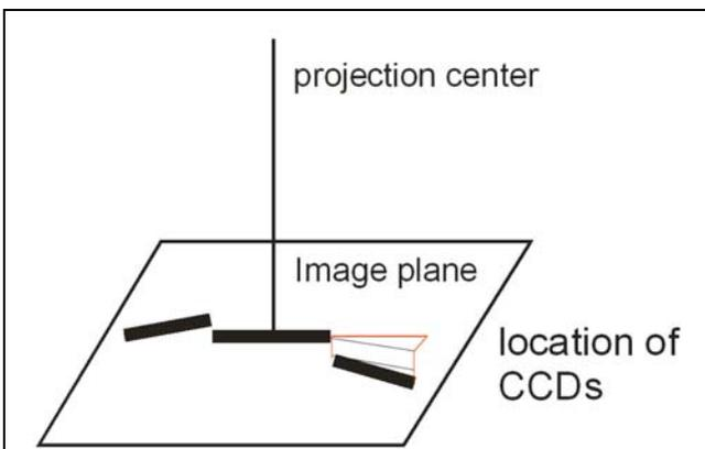
Fig. 5: location of CCDs in the focal plane – misalignment in the focal plane and vertical shift against the focal plane
