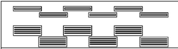
Fig. 1: arrangement of CCD-lines in focal plane of QuickBird
