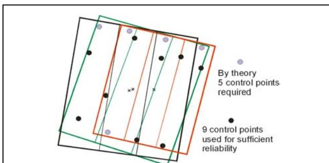
Fig. 9: IRS-1C scene and sub-scene configuration used for calibration – area Hannover
