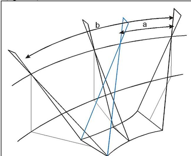
Fig. 15: slow down of imaging by permanent rotation of view direction slow down factor =  $b / a$
