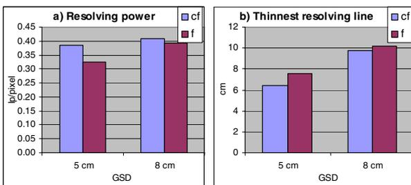
Figure 7. Determination of the spatial resolution from bar targets (f=flight direction, cf=cross flight direction). a) Resolving power and b) thinnest resolving line.
