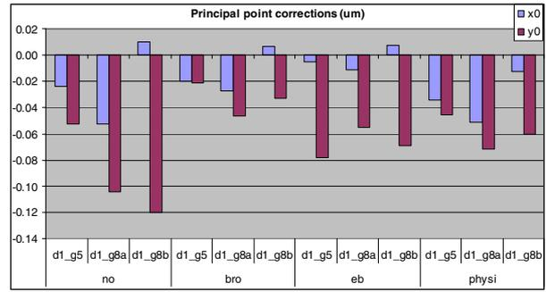
Figure 4. Corrections for principal point without additional parameters (no) with Brown's (bro), Ebner's (eb) and physical (physic) parameters.
