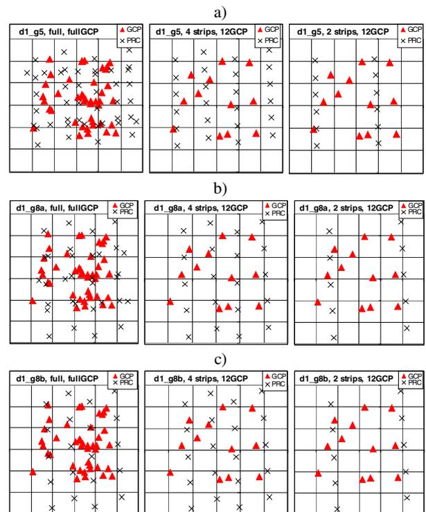
Figure 2. Block structures and GCP configurations at Sjökuilla large-scale test-field, approx. 40 GCPs. a) d1\_g5, b) d1\_g8a and c) d1\_g8b. Left: full block, full GCPs; Center: 4 strips, 12 GCPs; Right: 2 strips, 12 GCPs
