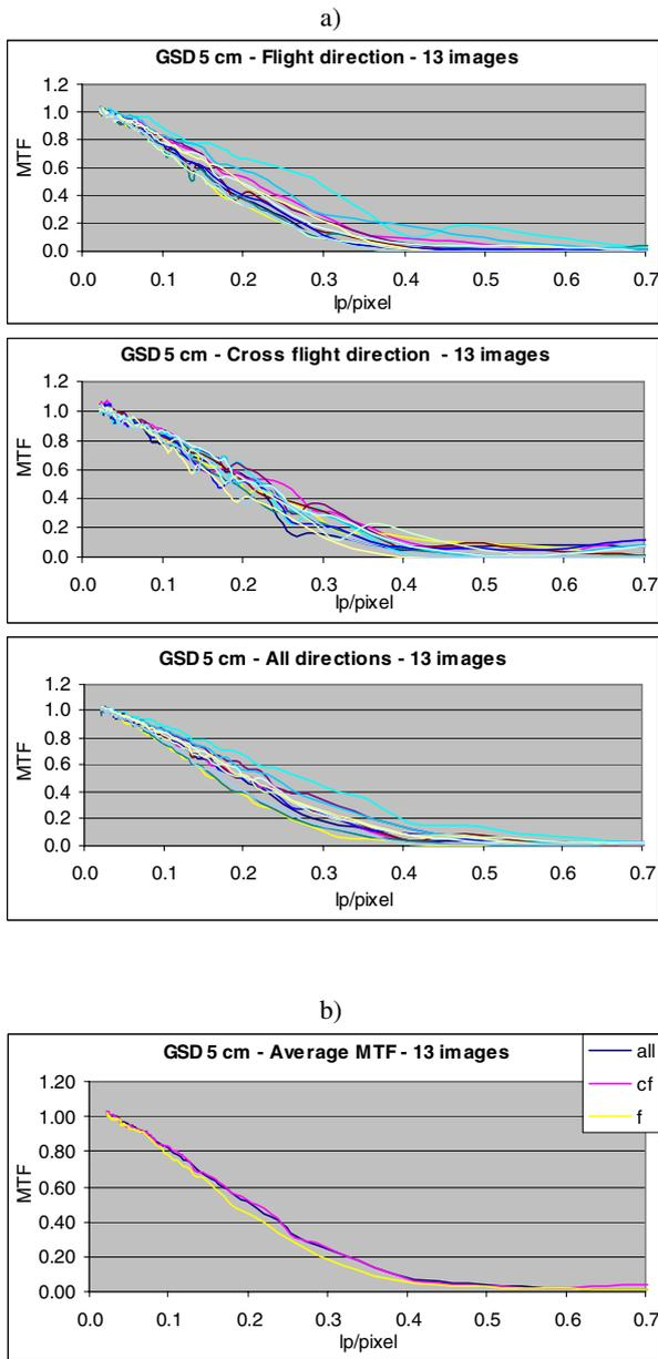
Figure 6. a) MTF of 13 images with 5 cm GSD in flight direction (top), cross flight direction (central) and the whole star (bottom), b) Average MTF of the 5 cm flight (f=flight direction, cf=cross flight direction).
