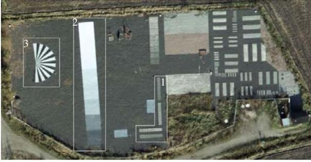
Figure 1. Overview of Sjökuilla test site. The test figures used in this study are: 1) permanent dense spatial resolution test bar targets, 2) transportable grey scale with 8 steps and 3) transportable Siemens star. Photo by Meixner.
