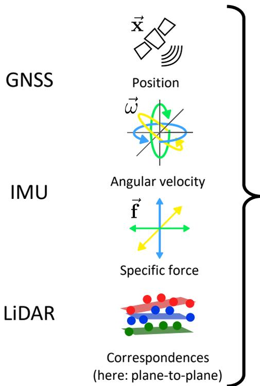
$$\underbrace{\tilde{p}}_{\text{measurement}} = \underbrace{x_{eb}^e(t) + R_b^e(t) (x_{bm}^b + R_m^b(t) x_{ma}^m)}_{\text{model}} + \underbrace{\epsilon_p}_{\text{error}}$$
