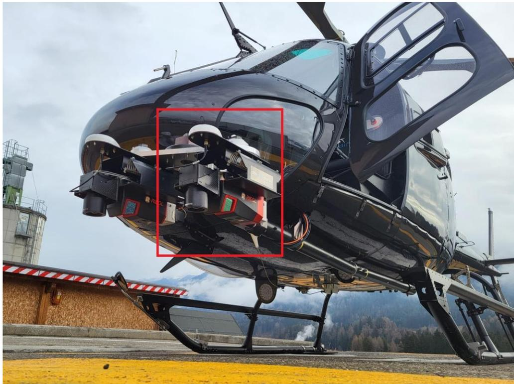
RIEGL VUX-160<sup>23</sup> with RiLOC-E-25 GNSS/IMU navigation system
